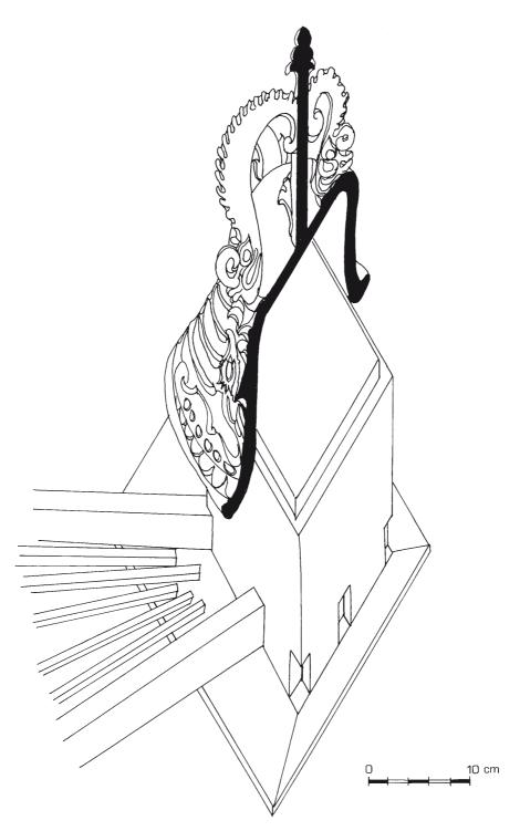
Fig. 72. Bali, implementation of a ridge finial over a radiating frame.
