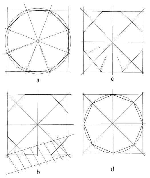
Fig. 1. Construction of an octagon, a, following the Mayamata, the method consisting of adding  $1/24^{\text{th}}$  of the side of the initial square, b, the method using  $3/7^{\text{th}}$  of the square, c, that using the average between the third and quarter of the square; finally, d, the usual construction in the west. The dotted lines of drawings a and c indicate, for comparative purposes, the exact location of the angles.
