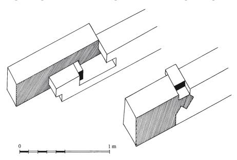
Fig. 13. Assembly of beams in a horizontal plane (line of Jupiter). The elements indicated in black represent the keystones, ensuring consistency.
