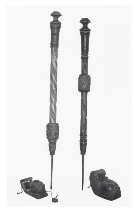
Ph. 6. Indonesia, Java and Sumatra. Archimedes drills (standing tools) and *riolet* wheels on the bottom.
