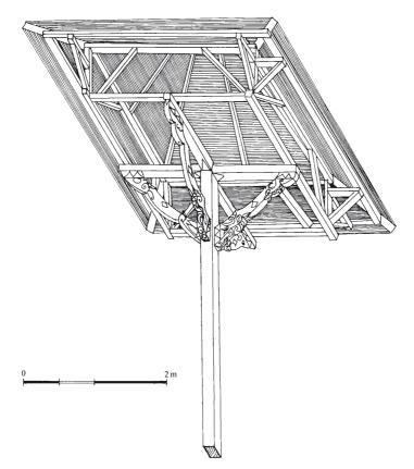
Fig. 30. Radiating frame over a central pillar in Java.
