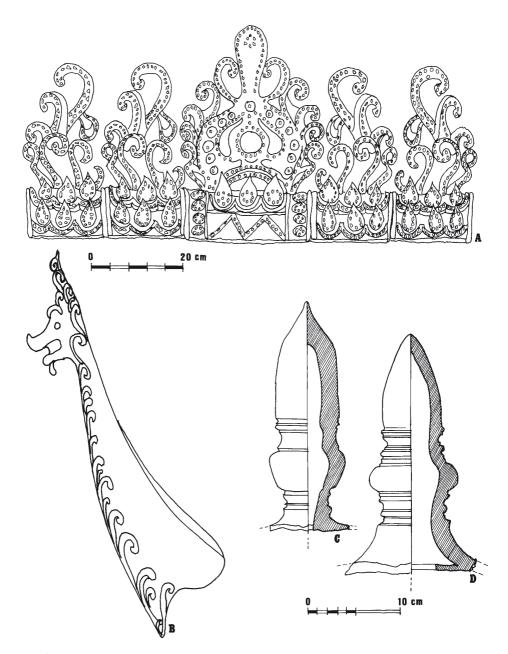
Fig. 73. Terra cotta roof siding: A, ridgecap of the Jepara region (Java). B, Chiang Mai, trim of the roof angle. C and D, Khmer ridge finials.
