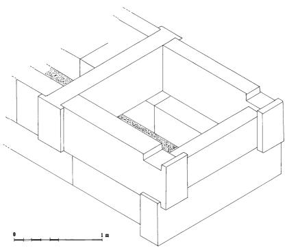
Fig. 77. Aukuna temple (Ceylon), assembly of the base of a double-sided wall, near the principal sanctuary door.
