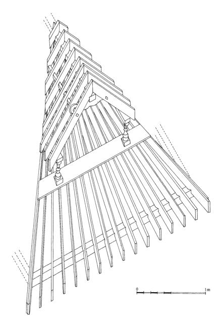
Fig. 25. Implementation of the frame of a false gable over a building covered with a radiating frame (Battambang region).
