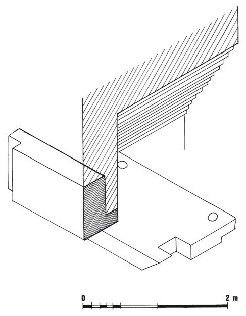
Fig. 66. Cambodia, brick discharge arch as a corbel.
