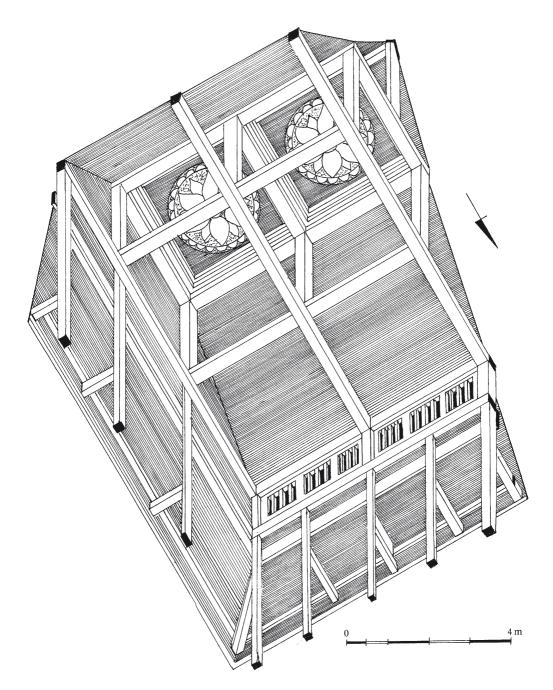
Fig. 23. Bending frame with partial ceiling and panelling, in Amarapura, Burma.
