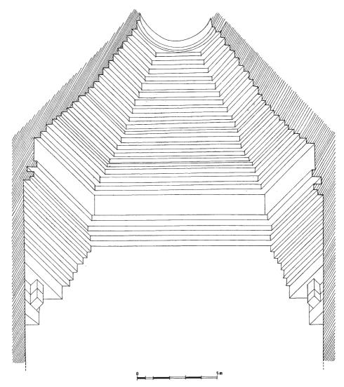
Fig. 83. Candi Kalasan, Java, passage from the square plane to the octagonal plane of the cella (corbel trumpet arches).
