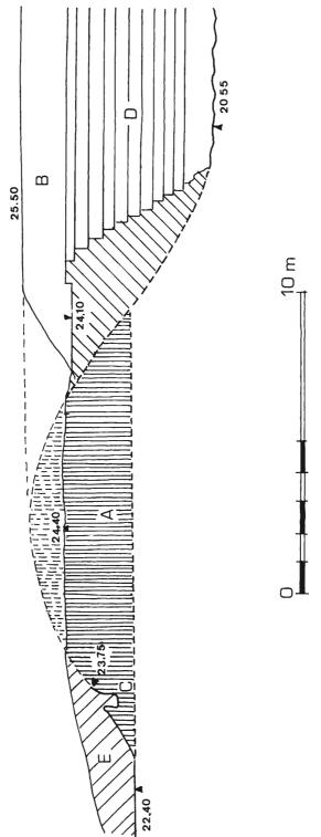
Fig. 94. Transformation of the Sras Srang, Cambodia. A, first state of the western excavation; B, first state of the northern excavation; C, canal of water distribution; D, second state of Sras Srang; E, excavated material after arrangement of second state.
