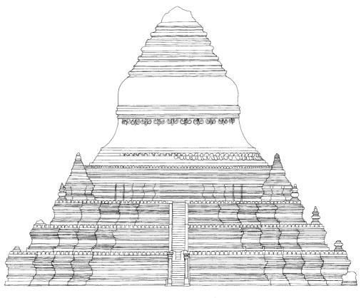
Fig. 62. Western elevation of the Mingalazedi stupa in Pagan (based on the photogrammetric information of the IGN).
