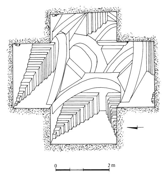
Fig. 61. Darasuram, axonometry of the intrados of the vault of the Amman temple cella.
