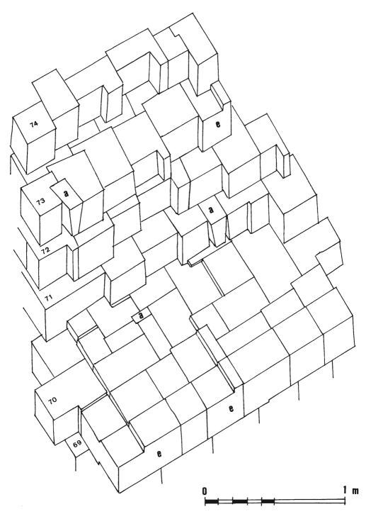
Fig. 81. Borobudur, stereotomy of the internal base on the level of the third gallery of the  $69^{\text{th}}$  to the  $74^{\text{th}}$  course, with striking wedge, and angle bar in the vertical plane (based on pl. LIII of *L'Histoire architecturale du Borobudur*, op. cit.).
