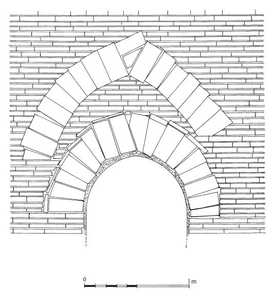
Fig. 65. Brick arch and its discharge, based on sketches made on site and photographs, in particular structure No. 484, Mingala-the-hpaya, Burma, of the inventory taken by P. Pichard, op. cit., vol. II.
