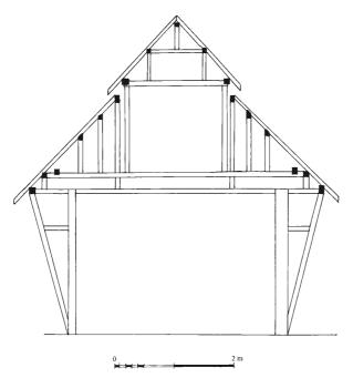
Fig. 26. Fragment of a bending frame with two sides over a structure with warped walls at Luang Prabang in Laos.
