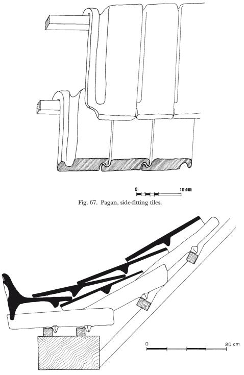
Fig. 68. Cambodia, restitution of the cut of a section of a sewer line in a  $12^{\text{th}}$  century Khmer roof.
