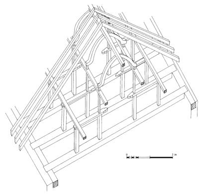
Fig. 27. Bending frame without crown post in the Darasuram region, India.
