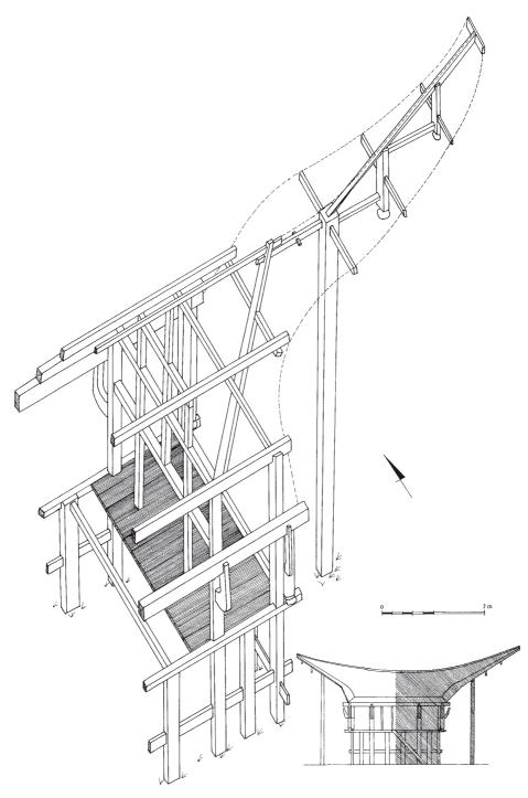
Fig. 35. Axonometry of the gable of a Toraja house (Sulawesi, Indonesia).
