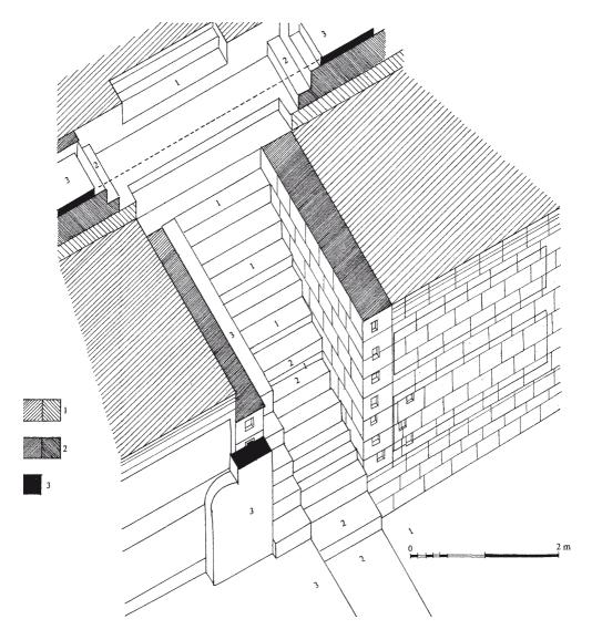
Fig. 92. Borobudur, repair of the second construction step, northern staircase from the first to the second gallery.
