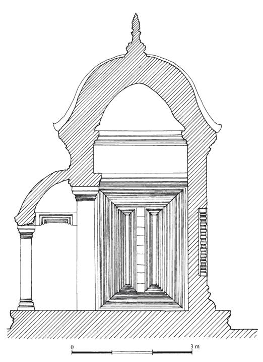
Fig. 45. Angkor Wat, false door with leaf, sculpted on the pavilion of the western entry of the exterior enclosure.
