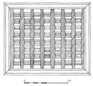
Fig. 41. Sandstone window of the fourth floor of Angkor Wat, outer side.
