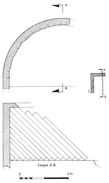
Fig. 56. Barrel vault constructed with unburnt bricks.
