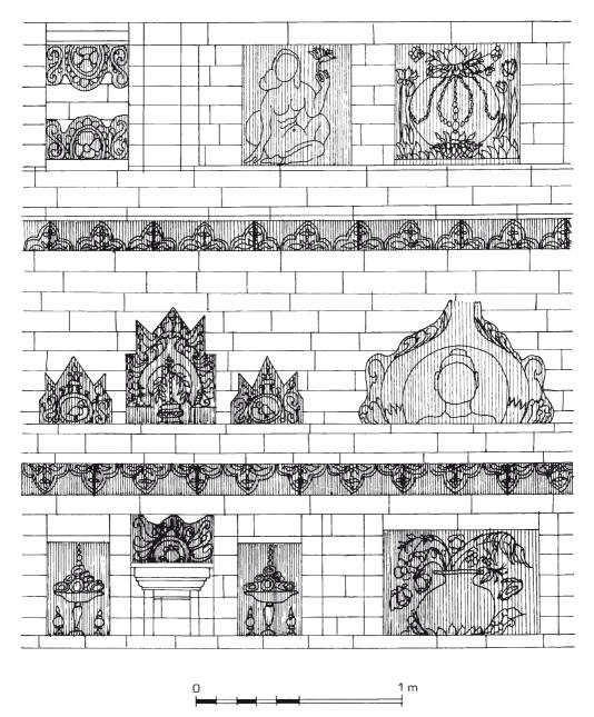
Fig. 89. Candi Gunung Gangsir, Java, detail of décor set into the brick bond of the base of the sanctuary wall; the different elements modelled into the terra cotta are hatched.
