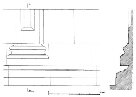
Fig. 74. Surkh Kotal, white lime siding of the foundation of the principal temple.
